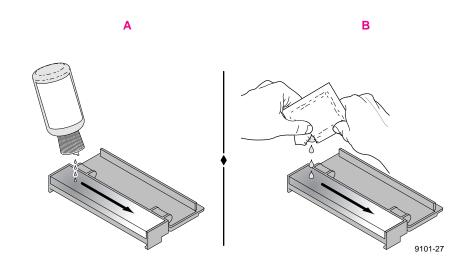
d. Place the cleaning tray in the media tray so that the tray's sponge pad is nearest the paper tray's handle. Press the two tabs underneath the cleaning tray into the two square notches provided in the media tray.
